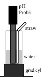
5. Insert the pH Sensor in the room temperature water. Also insert the straw so that it is fully below the water line. Begin collecting pH readings by tapping the Collect icon or pressing the Collect button. After
